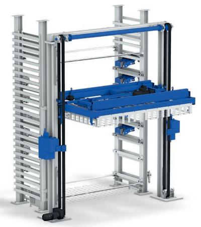
The PICKING TOWER by STOPA enables fully automated picking of raw sheets – perfectly tailored to your needs. Whether for individual production, for compiling and providing materials for processing machines, or for picking specialized customer orders: the STOPA PICKING TOWER efficiently and order-specifically sorts raw sheet packages.
